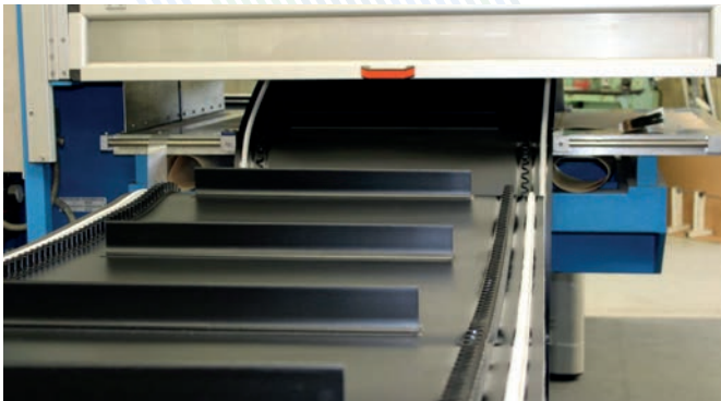
High Frequency welding of cleats
