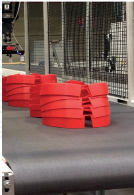
Low-noise fabric belt with fabric top cover for accumulation
